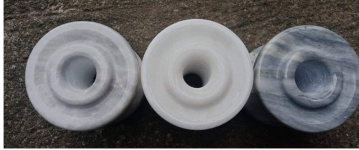
Figure 2. Various colored Marble Spool Insulators bearing the patent code PH 2/2020/050891.
