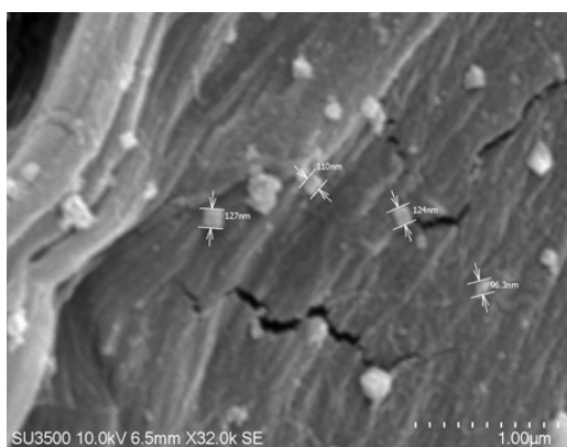
Figure 8. A magnified SEM image of the paper sensor showing an approximate AgNP particle size range of 96 nm to 127 nm.
