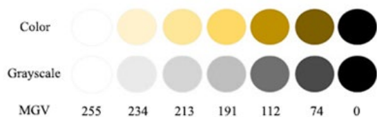
Figure 4. Sample shades of yellow brown converted to 32-bit grayscale image with equivalent MGV.
